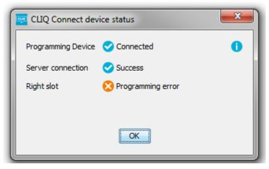
Programming error can occur when the key does not support direct programming (Generation 1 keys or Generation 2 keys with firmware below 12.1.0) or when the key had not been previously authenticated by a C-Key placed in the left port.
