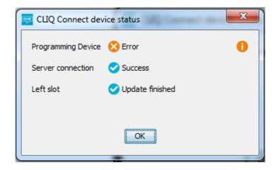
This problem may occur when computer and programming device are plugged into the docking station and USB port replicator. Sometimes after unplugging computer from the docking station, CLIQ Connect PC is indicating error status displayed on the screen above and there is "Port not found" information in logs. To solve this problem restart CLIQ Connect PC.
