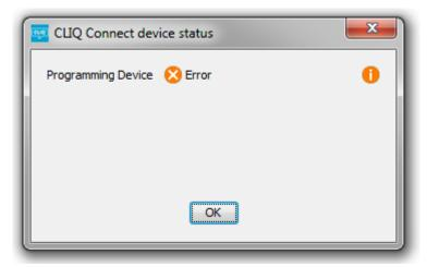
This may occur if another application connects to COM port of Local PD, preventing CLIQ Connect from doing the same. Make sure no other application is accessing the COM port assigned to Local PD when using CLIQ Connect.
