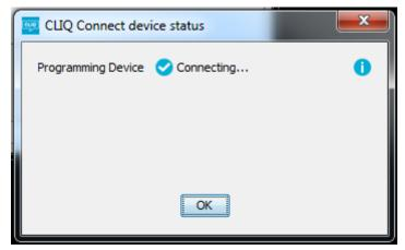
Connection between CLIQ Connect PC and Programming Device could hang just after plugging in Programming Device to a computer. Application icon in tray shows "connecting" status which looks like this:
